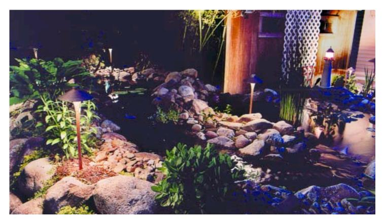
opportunity to add more lights. There are numerous methods to illuminating your pond. We do however discourage installing underwater lights in ponds. They will become covered with algae, can be hard to service, and are subject to corrosion. Also, for every foot of depth that the fixture is placed approximately 50% of the brightness or foot candles are lost. This lighting effect is murky at best. The following lighting design techniques will accentuate and enhance the natural beauty of any pond.
